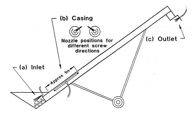
Figure 1 Alternative positions for liquid protectant spray nozzles
