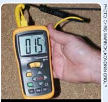
Deep temp testing: Dedicated temperature probes are ideal for testing grain temperature well below the surface. The basic alternative is a mercury thermometer fixed securely to a rod.
