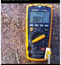
Multimeter temperature test: Higher grade multimeters can also test temperature. The one pictured includes a temperature wire as well as ambient temperature and relative humidity in addition to all the common multimeter functions used for electrical jobs around the farm.
