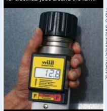
Moisture monitoring: A hand-held grain moisture meter is sufficient for monitoring stored grain. Be sure to calibrate it at the start of the season and record results to identify any change in moisture over time.
