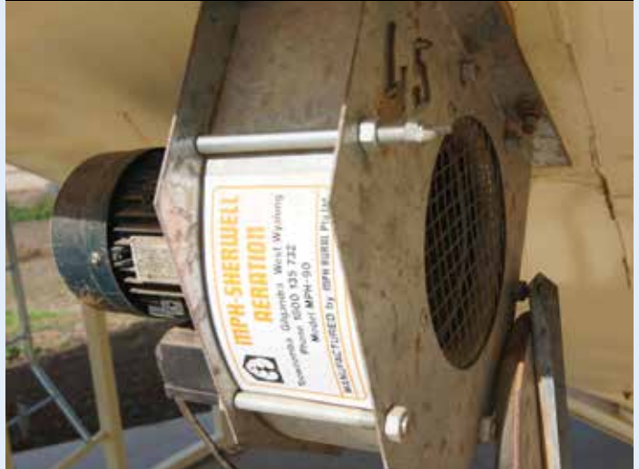
Small is sufficient: Aeration cooling fans on cone-bottom silos typically only require 0.37kw (0.5hp) electric motors.
