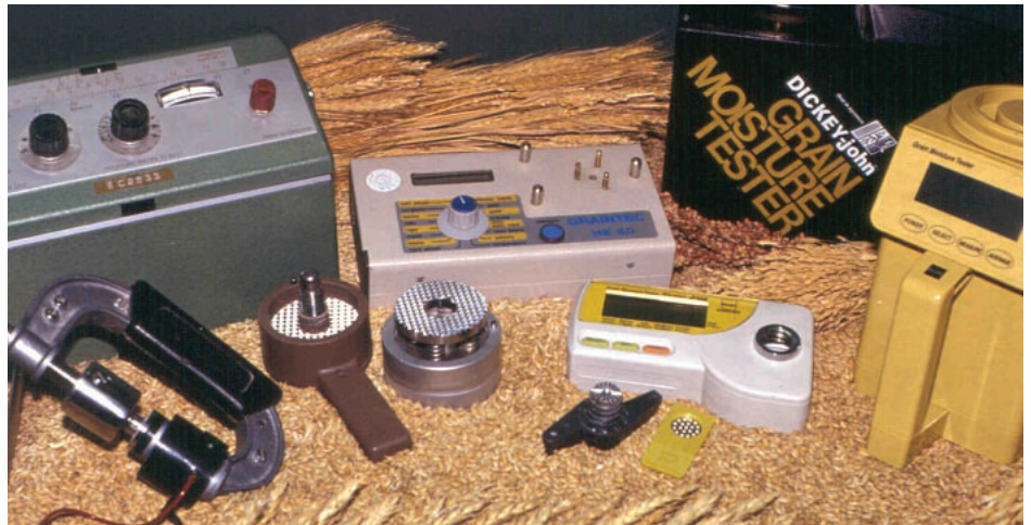
There is a range of portable conductance and capacitance meters available to measure grain moisture in the paddock. The moisture meters all need to be calibrated and used in a consistent manner to enable accurate moisture measurements.
