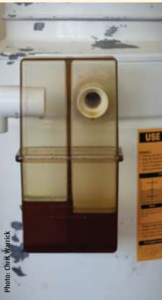
Relief: Oil relief valves allow for air expansion and contraction in a sealable silo and double as a pressure-test gauge.
