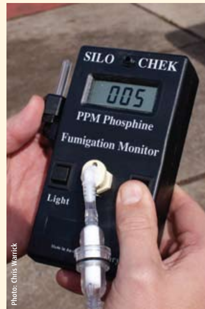
Phosphine: Before fumigating, tubes can be inserted into various positions within a sealable silo. A phosphine meter can then be connected to the tubes to monitor the concentration levels of phosphine during the fumigation period.
