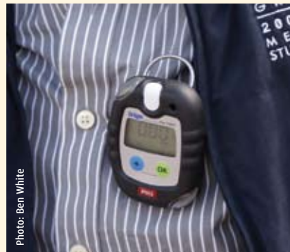
Safety: A personal safety monitor like the one pictured will sound an alarm when it senses phosphine levels that are potentially dangerous to humans.
