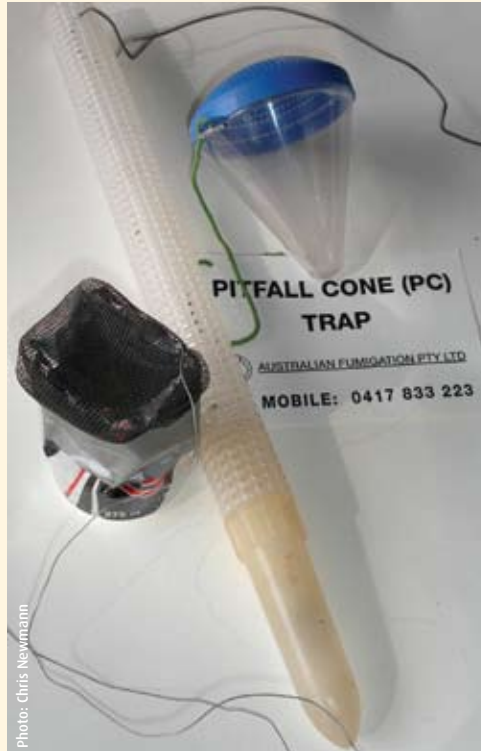
Traps: Insect traps are an efficient monitoring tool. Push whole probe or pitfall cone trap just below the surface of the grain to capture insects moving through grain and inspect traps at least monthly.
