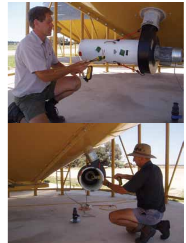
Figure 2: The 'A-Flow' fitted to the aeration fan intake ready for air flow measurements.
