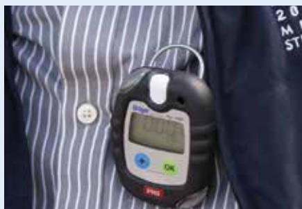
Life saver: Personal phosphine monitors sound an alarm if harmful concentration levels are detected.
