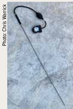
A low-level phosphine meter is the surest way to know if grain has been adequately vented to the delivery requirements.
