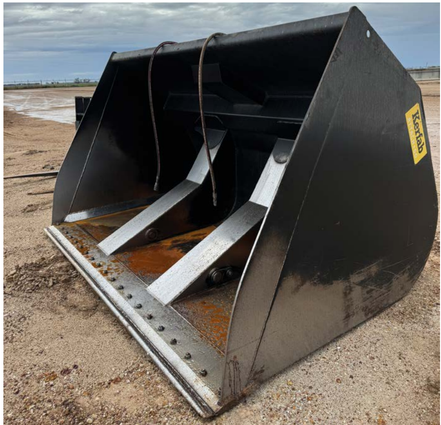
The Kerfab outload loader bucket holds 6m 3 heaped.
