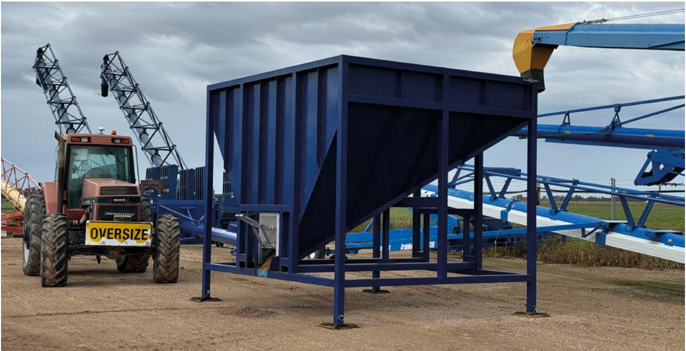
Grain blending from the bunkers comes through these blending hoppers.
