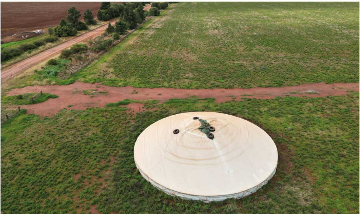
Placement of the ring close to the road for ease of outload.
