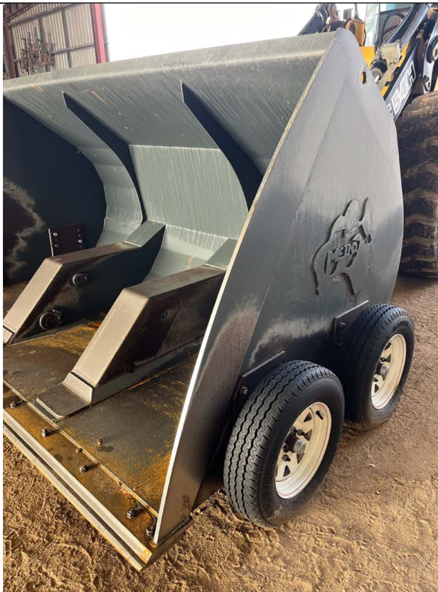
Keeping ground tarps in one piece is made easier with the addition of wheels on the bucket and a fork-mounted broom. Photo: Sam Heagney
