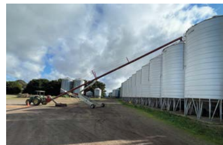
A swing-way auger helps with unloading duties in the shed as well as loading silos.
