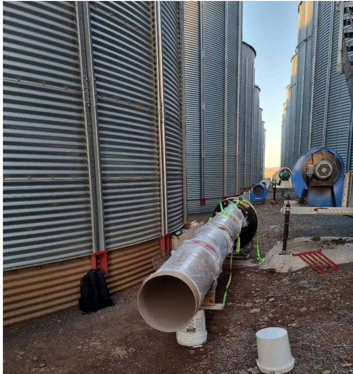
Figure 2: Airflow measurements were taken at the fan inlet to evaluate the accuracy of the Schmelzer meter to measure total airflow through the silo.
