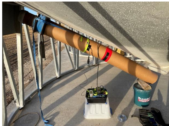
Figure Group 1: Measuring airflow using a pipe on the fan inlet, so backpressure readings could be recorded relative to airflow.
