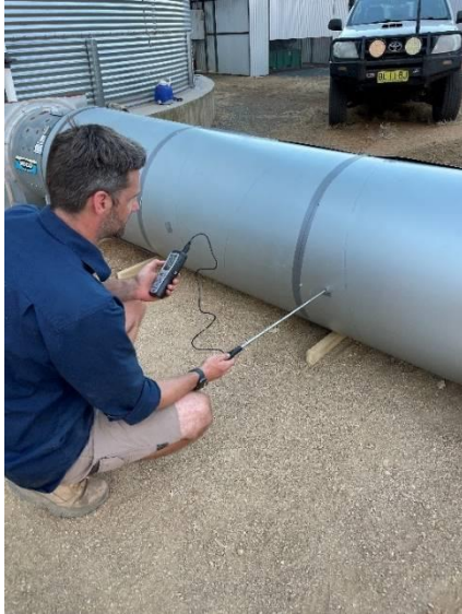
Image 2: Hotwire anemometer used to take airflow measurements.
