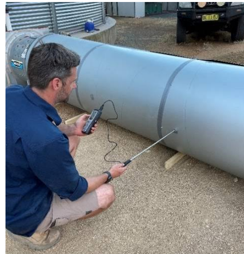
Figure 9: Hotwire anemometer used to take airflow measurements.
