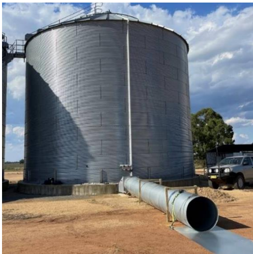
Figure 8: Pipe on fan inlet to measure airflow while silo was full of canola.
