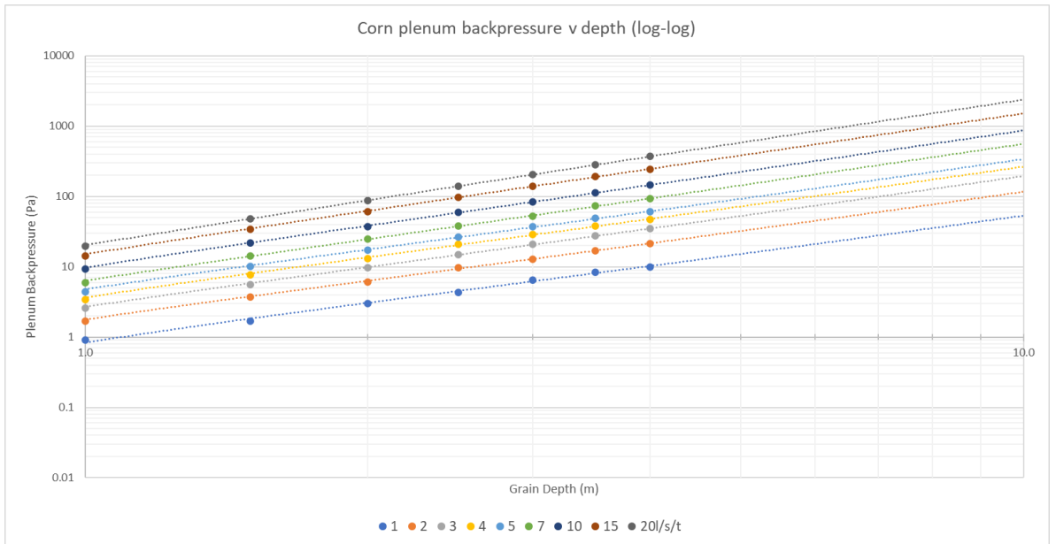
Figure 21: Logarithmic corn plenum backpressure with depth at 1-20l/s/t airflow.
