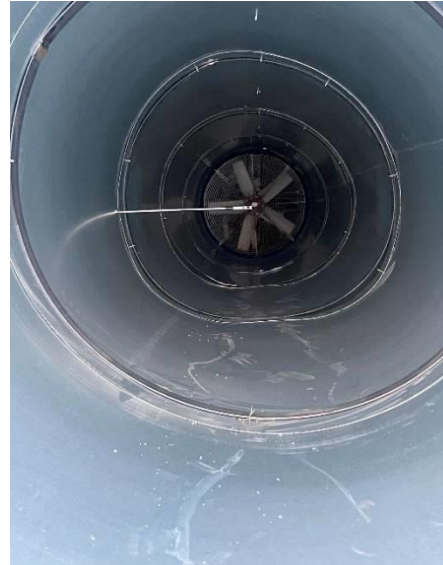
Image 3: Hotwire anemometer reading at seven places across the diameter of the pipe.
