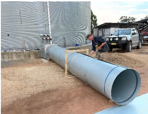
Figure Group 1: Measuring airflow using a pipe on the fan inlet, so backpressure readings could be recorded relative to airflow.
