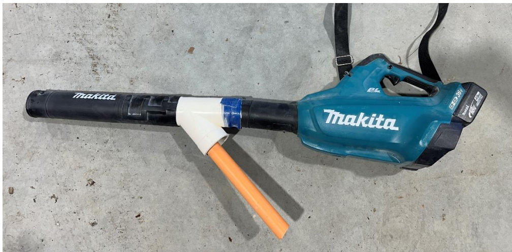
Figure 1. Home-made venturi fitted to a 36volt leaf blower used to apply the DE.
