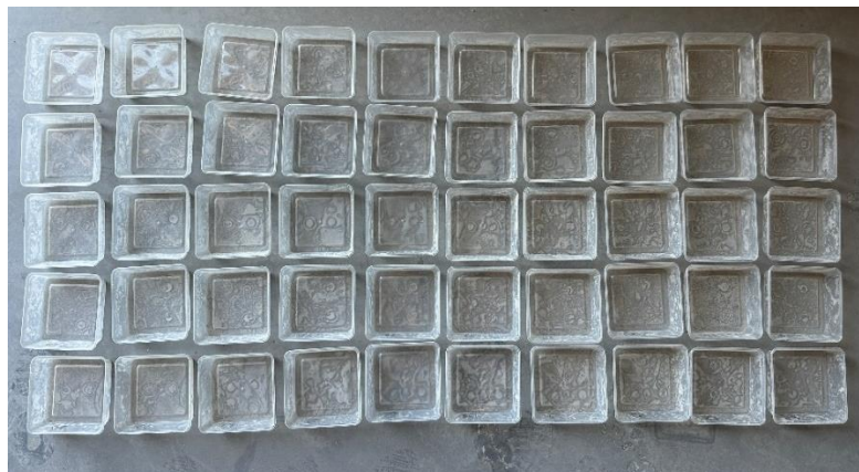
Trays collected after weighing for visual assessment of dust quantity in each.
