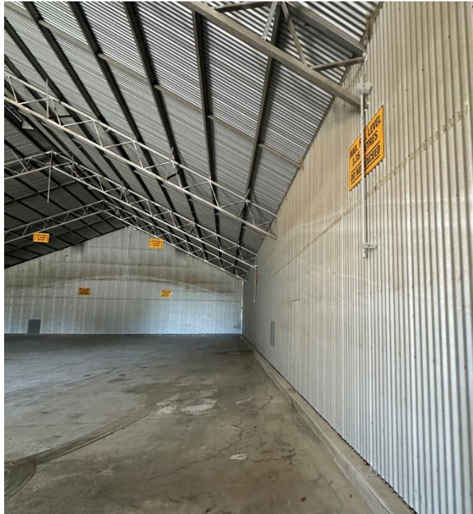
Some of the tray positions used to collect DE dust for measurement, (floor beside the wall, halfway up the wall and at the top of the wall).
