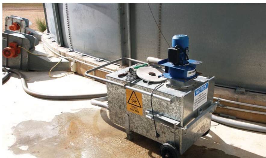
Photo 10: Powered recirculation improves gas distribution through a gas-tight sealable silo enabling 7-10 day exposure rather than 20-day exposure when fumigating silos greater than 300 t capacity. (Source: Chris Warrick, Primary Business)
