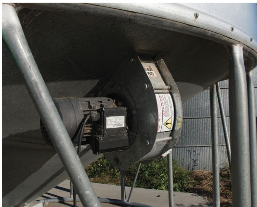
Photo 15: Aeration cooling is essential for storing oilseeds and may require higher-capacity fans to achieve airflow rates of 2-3 L/s/t in small-seeded crops such as canola. (Source: Chris Warrick, Primary Business)
