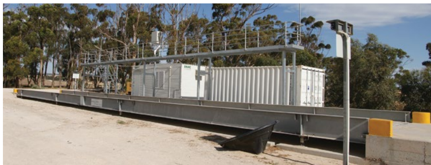
Photo 9: The addition of a weighbridge can help maximise truck carrying efficiency and avoid overloading fines. (Source: Ben White, Kondinin Group)
