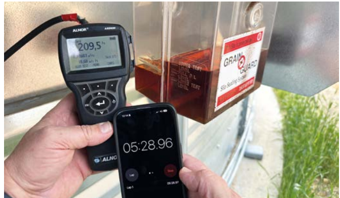
Good times: Kondinin Group researchers together with the Grain Storage Extension Team tested cone-bottom and flat-bottom silos across the country to check for Australian Standard sealing compliance. Photo: Chris Warrick
