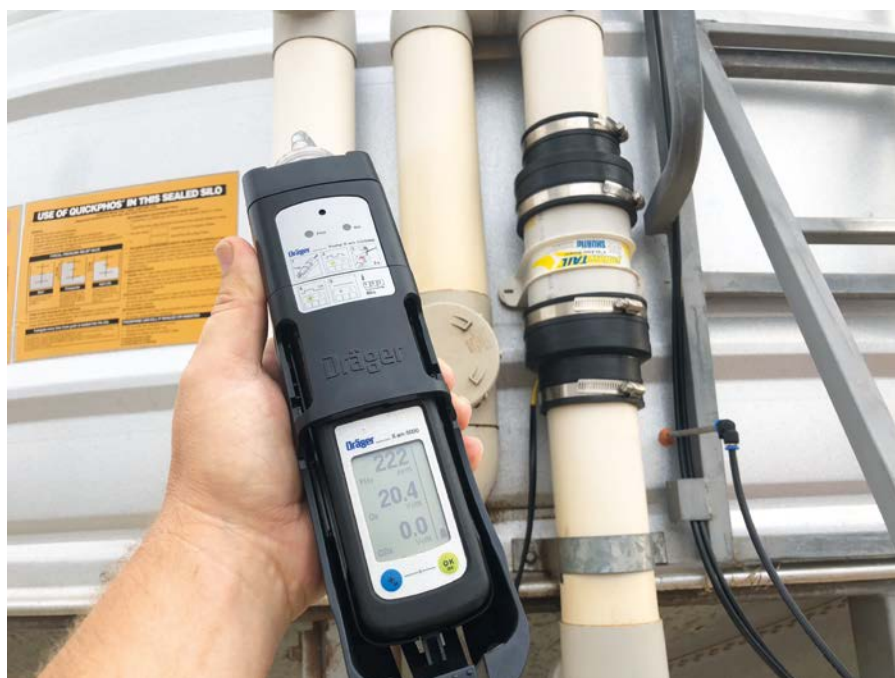
Monitoring tool: High-range meters like this Dräger X-am series can measure achieved concentrations during fumigation.
