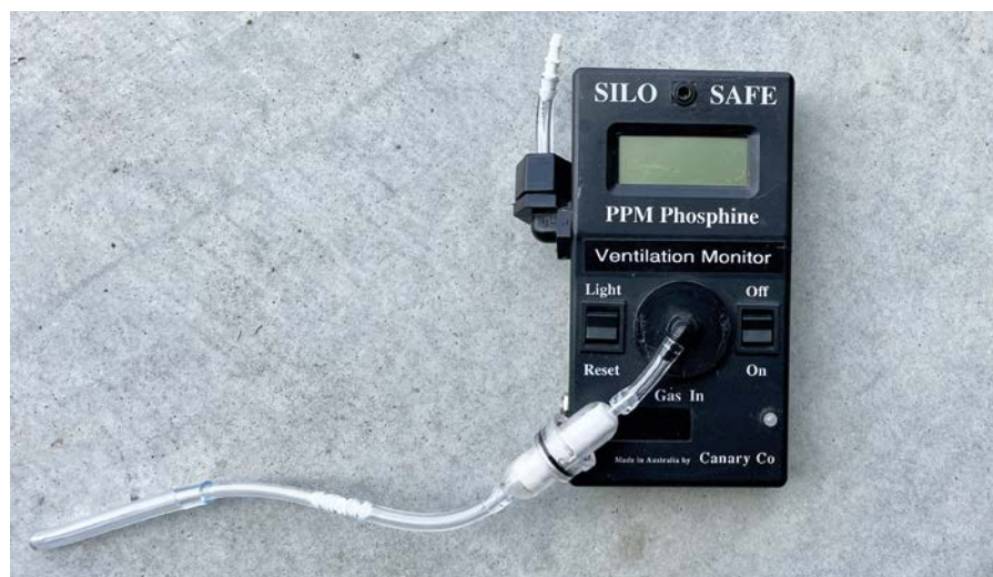
Clearance confidence: A low-range meter like this Silo Safe from the Canary Co can provide confidence grain has been adequately ventilated after fumigation. Photo: Chris Warrick
